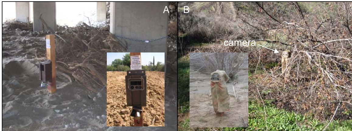
Figure 6. Camera station designs for units placed under bridges with steel box and chain (A), and cameras deployed without steel box and concealed with burlap (B).
